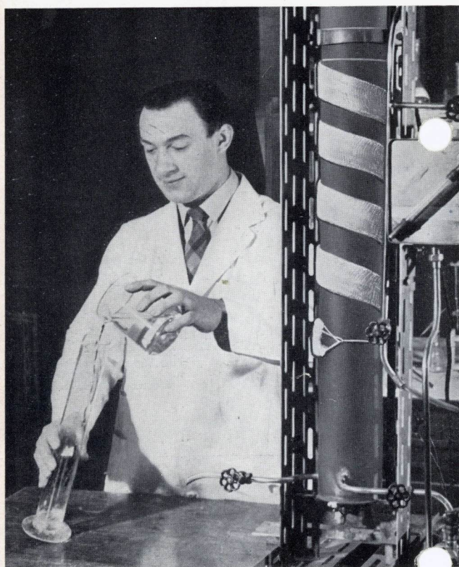
A heating tape used on an experimental copper counter-flow ring-packed column, running at elevated temperatures.
